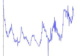
Sensors may contain circuits that smooth the data before you ever get to see it. If not, data logging software has various ways to remove noise. Borrowing from the world of electronics, it may offer different smoothing algorithms: the median smoothing algorithm simply averages readings that are close together while Fourier smoothing looks for high frequency changes. For example, you could remove a sudden spike in a graph with Fourier smoothing, when averaging would leave the graph with a bump.
